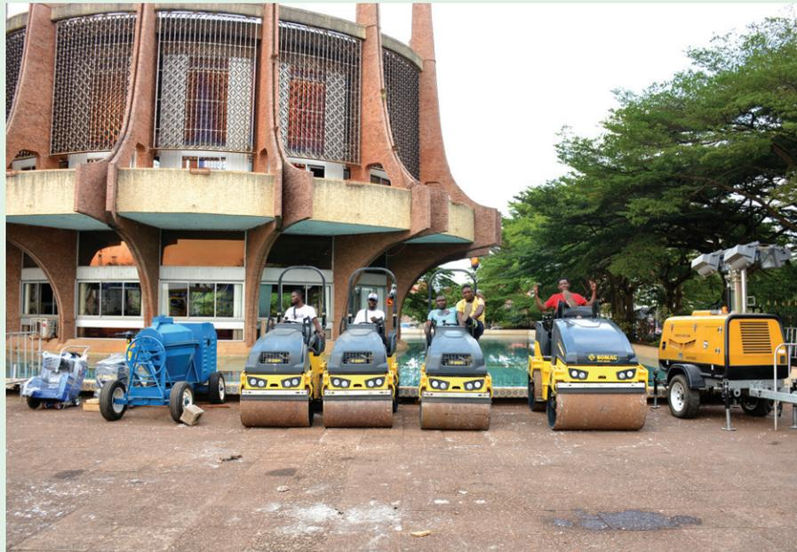
Council, the mayor revealed, recently purchased equipment. They included two medium BOMAG compactors (single drum rollers designed for compacting mixed soils and cohesive soils in thin to medium layers), and two mini compactors.
